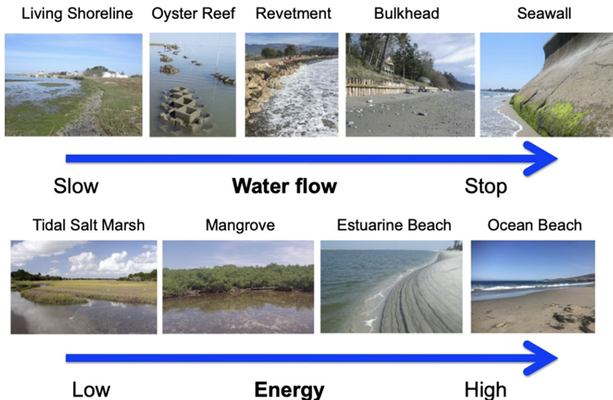
Fig. 12 Illustration of gradients in the two axes of influence for the conceptual model of shoreline armoring effects. Top row: Engineering purpose with respect to intended effect of structure on water flow (slow vs. stop). Bottom row: Hydrodynamic energy (low to high) at the structure as determined by the environment. Adapted from Dugan et al. (2018) .
